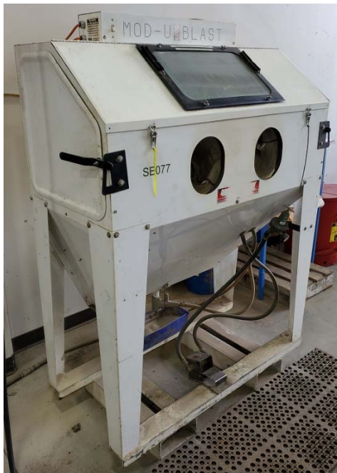
Mod-U-Blast Cabinet Abrasive blaster – Used for small parts and components
